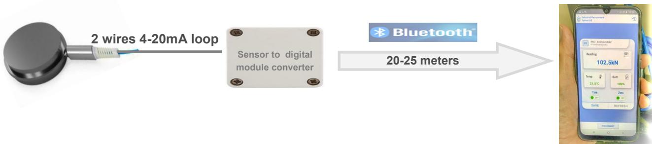
This smart and advanced battery-operated sensor converter, will turn any sensor with two (4-20mA) wires to become “smart” digital sensor with Bluetooth communication. Free Android Apps for continually reading the sensor by smart phones (or tablets) and saving the readings to history file in excel format. File than can be send directly from the phone to any email or as a message.
